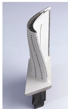
Fig. 1. Recent film-cooled high-pressure turbine blade covered with ceramic TBC coating [4]
