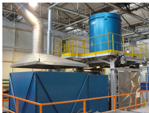
Fig. 10. Bell-cover with boxes before loading to VPA furnace
