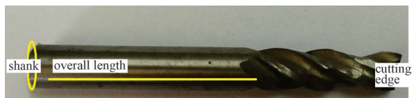
Fig. 1. Nomenclature of cutting tool
