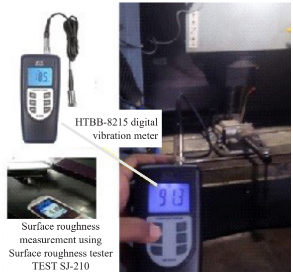
Fig. 3. Measuring devices: vibration meter and surface tester SJ-210
